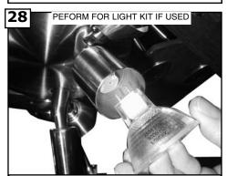
Plug in the 3 light bulbs by aligning the 2 prongs on bulb with holes in socket and then push in and twist the 50 watt bulbs which are GU10.
